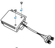
5. Secure the front of the metal cover with the long screw that you removed in step 2
